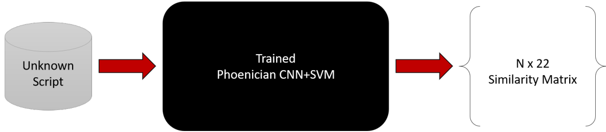
Figure 10: The predictive CNN+SVM classifier comparing the other seven scripts to the Phoenician alphabet. The unknown script is replaced with any of the seven other scripts. The size of the matrix is dependent on the number of symbols in the unknown script provided.
